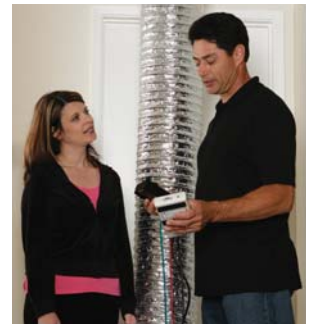
Air Duct Pressure Testing pinpoints leaks that can lead to higher energy bills and lower efficiency.
